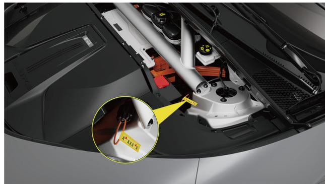
4. Find the low-voltage MSD in bonnet and remove it, and the vehicle will deactivate the high-voltage system automatically.
