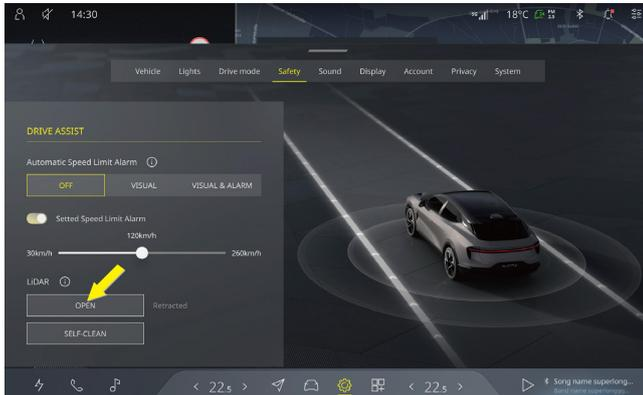
When the vehicle is powered on and the gear lever is engaged in Park (P) gear, all lidars can be manually deployed with one click as needed. If any of the following situations occur, it is not possible to manually deploy the lidars:
