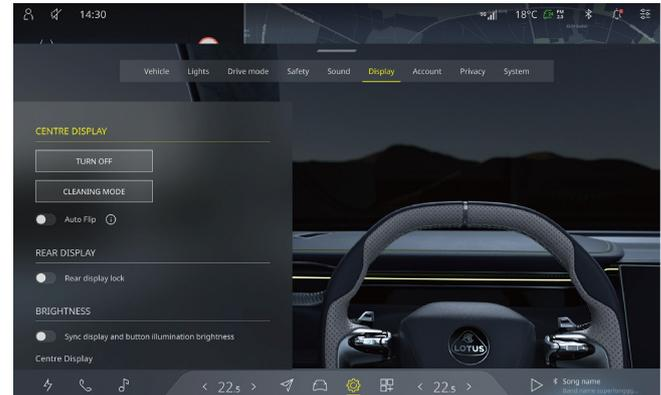
On this interface, you can turn off the CSD, cleaning mode, auto flip, brightness and HUD.
