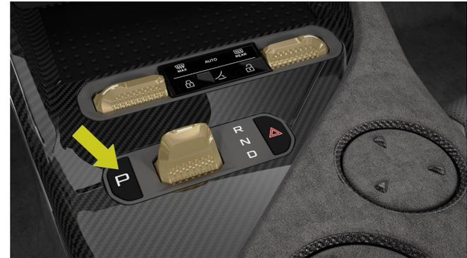
After the vehicle is parked, press the P button, the gear switches to P gear, and the electronic parking brake is automatically activated.
