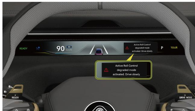
When a fault alarm related to the Lotus intelligent anti-roll control system is displayed on the instrument cluster, you are not allowed to drive on rough roads and turn at low speed. In this case, contact the Lotus Customer Care Centre in time to eliminate the fault.
