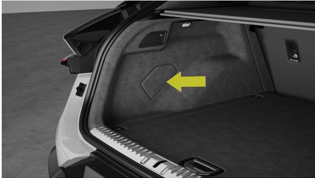
Remove the boot storage box to find the rear electric fuse box.
