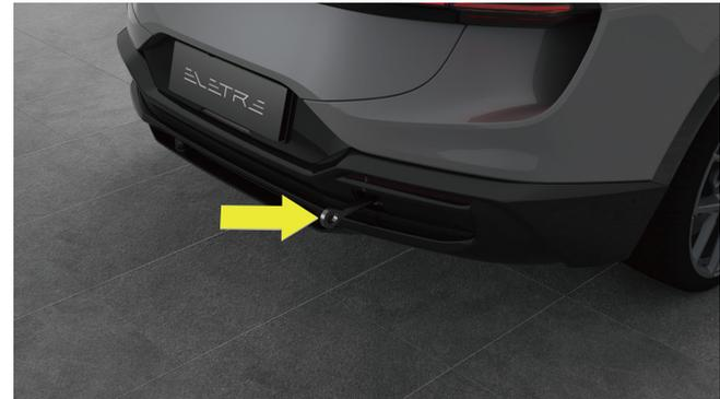
4. Screw the towing eye in place and continue tightening until the towing eye is fully screwed in and the towing device is attached to the towing eye.
