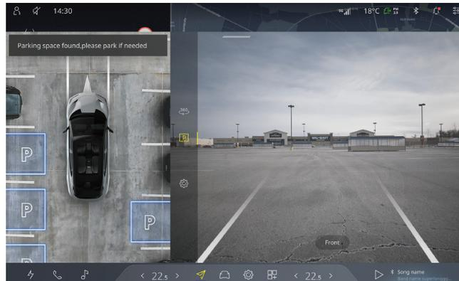
3. If an available parking space is found, depress the brake pedal to stop the car stably and click the **IN CAR** button.
