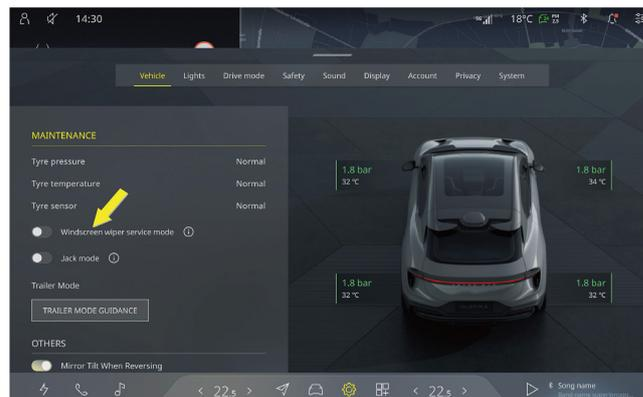
Before replacing the front wiper blade, please click on the **Setting - Vehicle - Windscreen wipers service mode** in the centre display, and the front wiper arm will be moved to the service position.
