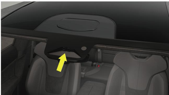
The microwave window is fixed horizontally in the centre, vertically upward position of the front windscreen. Information about the vehicle is stored in the microwave window. Please keep the front windscreen clean and prevent foreign objects from blocking the microwave window.
