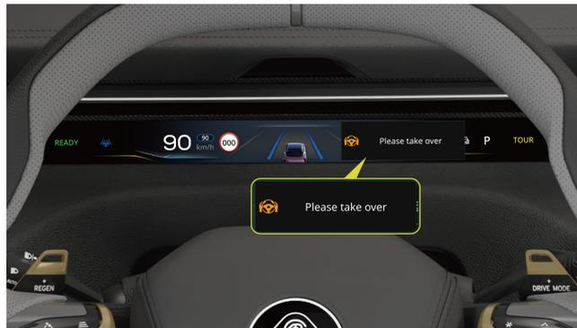
When the HWA is working, if the system detects that the driver is not holding the steering wheel, it will display on the combined instrument to take over the vehicle text prompts, accompanied by overriding prompt tone. If the alarm is ignored, the HWA will exit.
