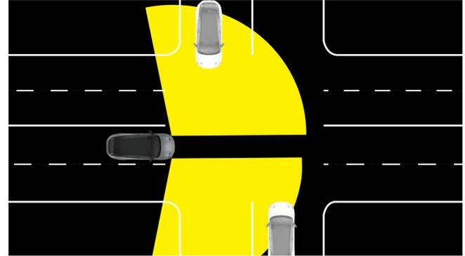
When you are driving out of the parking space or passing an intersection, if FCTA detects that there is a risk of side collision in the front, it will remind the driver to pay attention to the side oncoming vehicles. When necessary, automatic emergency braking will be applied to avoid or mitigate the collision.
