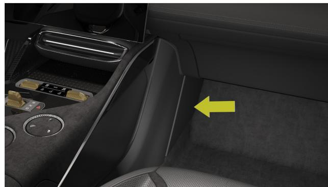
The central fuse box is located on the right side of the tunnel console, which can be viewed by removing the right front bezel of the tunnel console.
