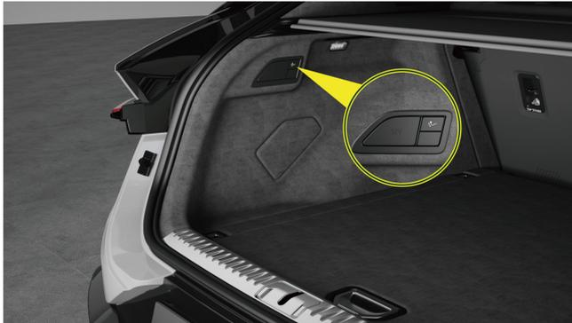
1. Open the tailgate, press the electric towing hook switch located in the boot. The electric towing hook will extend automatically.
