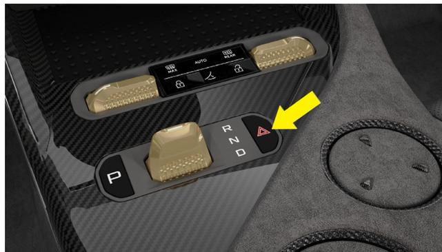
In case of emergency during driving, please press the hazard warning light switch button to activate the hazard warning lights.
