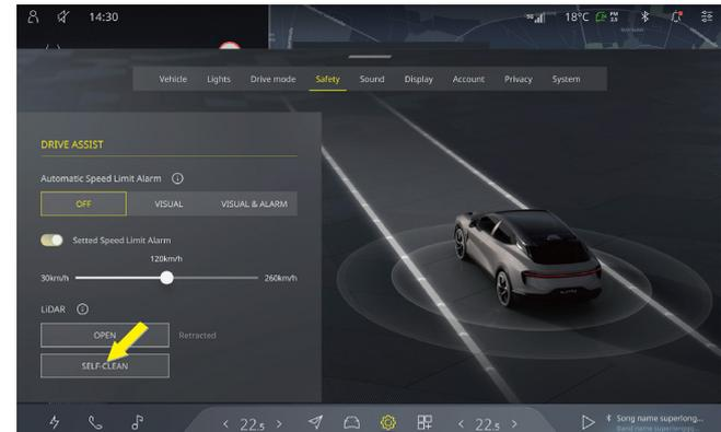
When the vehicle is powered on and the gear lever is engaged in Park (P) gear, all lidars can be manually cleaned with one click as needed. If any of the following situations occur, it is not possible to manually clean the lidars:
