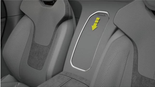
The rear seat backrest pocket is located in the centre of the rear seat backrest, and is pushed down to the bottom lock; Press again and close automatically.
