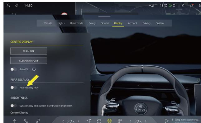
When you turn on the **Rear display lock** switch, clicking the rear display will briefly light up the screen and prompt you to restart the rear display. If you do not perform any operation, after a period of time, the rear display will automatically screen.
