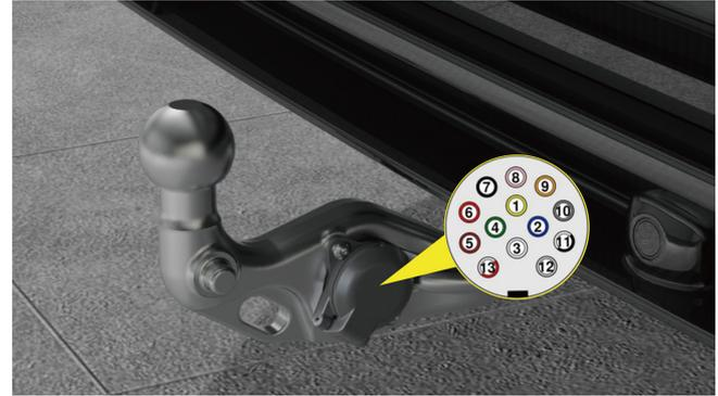
After the protective cover is opened, it can be used. The electric connector equipped with this vehicle adopts a 13-core coil, and the standard used for the power outlet is ISO 11446:2004. The specific pin functions are as follows:
