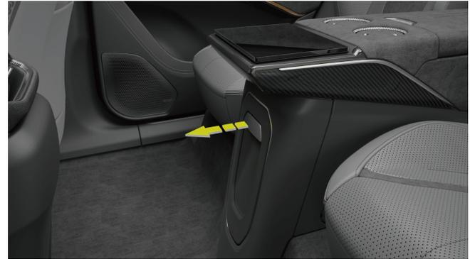
The rear tunnel console pocket is located under the rear seat centre armrest, which can be opened by pulling it out.
