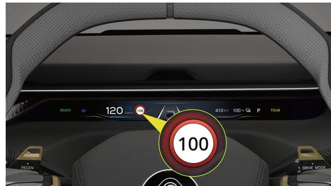
The alarm will be triggered when the vehicle speed exceeds the speed limit recognized by the system; The alarm will be released when the vehicle speed is below the speed limit recognized by the system until a new speed limit is detected.
