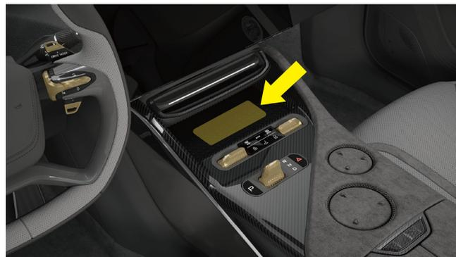
The driver can unlock the vehicle with the key fob/NFC digital key and get inside, and depress the brake pedal within 2min to start the vehicle. If the vehicle is not started within 2 minutes, the CSD will give a prompt accordingly. At this time the key fob/NFC digital key needs to be put in the wireless charging induction area. Then the
