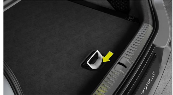
Additional pocket is provided under the boot floor, which can be used to store the charging equipment in the vehicle.
