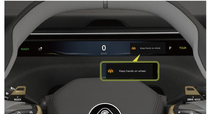
When LKA works, the driver is required to hold the steering wheel with both hands at all times. When the LKA is activated for the first time and the system detects that the driver is not holding the steering wheel, no prompt message will appear on the instrument cluster. If the LKA is activated again in the next period of time, and the system detects that the driver is still not holding the steering wheel, it will prompt "Please hold the steering wheel" on
