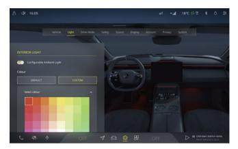
This screen allows you to set up external and internal lighting.
