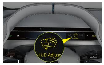
Swipe the right multifunction key left and right to set HUD on or off, adjust height and angle, brightness, and snow mode.
