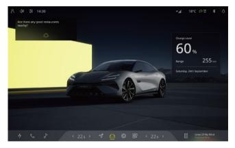
To wake up the voice function, you can say the wake-up words ("Hi, Lotus" or "Hello, Lotus" by default) or press the voice button on the right side of the steering wheel. When the voice function responds to your wake-up, a voice broadcast bubble will appear in the CSD.
