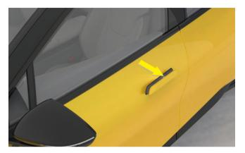
When the ambient light outside the vehicle is insufficient, the handlebar light will be illuminated to illuminate the inside of the door handle for the convenience of vehicle unlocking, and then it will be automatically extinguished after a period of time.
