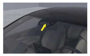
The microwave window is fixed horizontally in the centre, vertically upward position of the front windscreen. Information about the vehicle is stored in the microwave window. Please keep the front windscreen clean and prevent foreign objects from blocking the microwave window.
