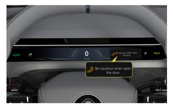
If DOW detects a target and there is a risk of collision when the door is being opened, the indicator on the outside mirror will be illuminated or flash, accompanied by an audible alarm, and images and text alarm signals will pop up on the instrument cluster.
