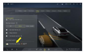
The passenger front airbag is turned on by default, and when the front passenger seat has a reverse-mounted child seat, a vehicle crash can cause personal injury and unnecessary financial loss when the airbag pops out. When installing the child safety seat in the passenger seat, be sure to click the icon in the centre stack display and select Safety to manually turn off the front passenger airbag.
