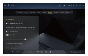
Click the  $^{\textcircled{0}}$  icon on the CSD and click **Display** to access the display brightness setting interface. Then click to turn on or off the auto adjustment.
