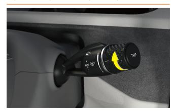
The sensitivity of the induced rainfall can be adjusted by turning the sensitivity scroll wheel of the RLSM upward and downward. The higher the sensitivity when turning the scroll wheel upward, the shorter the wiping interval will be. Conversely, the lower the sensitivity when turning the scroll wheel downward, the longer the wiping interval will be.
