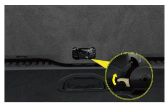
Emergency unlocking of tailgate control lever
