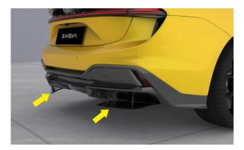
The active rear diffuser can be found under the rear bumper. When the vehicle speed is greater than 90km/h, the active rear diffuser will be automatically turned on. When the vehicle speed is lower than 30km/h, the active rear diffuser, if turned on, will be automatically turned off.
