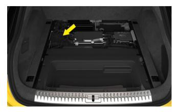
Remove the boot storage box to find the rear main distribution fuse box.
