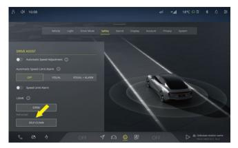
When the vehicle is powered on and the gear lever is in the P position, the front LiDAR can be cleaned manually with one touch as needed. The LiDAR cannot be cleaned manually in any of the following conditions:
