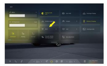
Click the  $\frac{\circ}{\circ\circ\circ}$  icon in the CSD to open the Wi-Fi setting interface. Enable the Wi-Fi network and activate the hotspot function in your phone, then you can find your phone's hotspot name in the **Networks Found** . Click connect, and the Wi-Fi network setting is completed.
