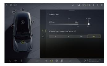
Tap the  $\square$  icon on the central stack display and select the charging APP to access the charging setting interface.
