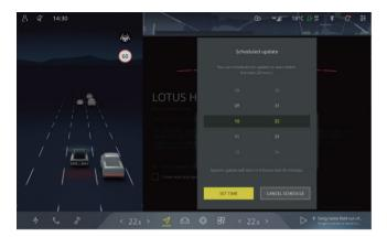
You can also schedule an OTA system upgrade at any time within 24 hours. Once set, the scheduled upgrade icon will be displayed at the upper right of the interface. The system will automatically start the OTA upgrade at the scheduled time when the network is connected.
