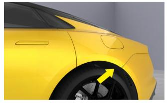
2. Push the charging port cover lock lever backwards to unlock the charging port cover, pull it out from the gap and open the charging port cover.
