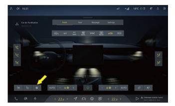
Tap the temperature value in the CSD to switch to the A/C control interface, then tap the  $\oplus$  icon to turn on the steering wheel heating function at level 3 by default. Repeat taps on the level to lower the level further until the heating function stops.
