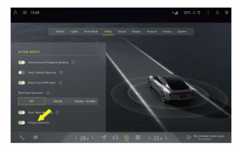
Click the @ icon on CSD, and select **Safety** to switch to the setting interface, where you can click to turn **Fatigue detection** on or off.
