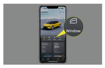
Tap the window switch on the mobile APP to fully open or close the windows. Before the full opening or closing of windows, the windows will not stop moving even if you tap the window switch on the mobile APP again.
