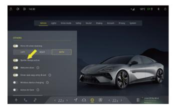
Click the icon on CSD and select **Vehicle** to open the **Spoiler always active**, when the spoiler always active is turned on, the active rear spoiler of the vehicle will remain in the position set before the power is turned off. When the spoiler always active is closed, the active rear wing of the vehicle will automatically turn off.
