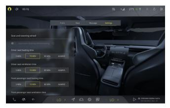
Tap the **Settings** in the A/C control interface on the CSD to switch to the front seat heating setting interface.
