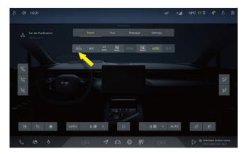
Click the **TEMP** in the CSD to switch to the climate control interface where you can activate or deactivate the defrosting/defogging function of the streaming mirror to remove rain, water mist or ice and snow from the camera.
