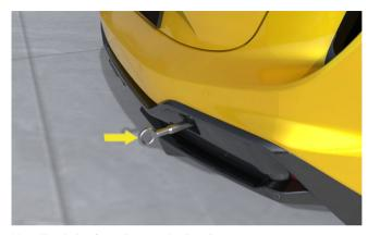
Mounting hole of rear bumper towing ring
