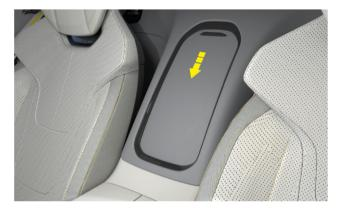
The rear seat backrest pocket is located in the centre of the rear seat backrest, and it can be locked should it be pushed down to the bottom and will close automatically should it be pressed again.
