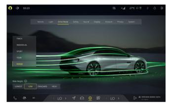
In this screen, you can set the driving mode, and in some driving modes, you can set the body height. The driving mode includes track mode\*, individual mode, sport mode, tour mode, range mode.
