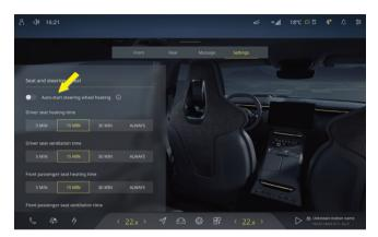
You can tap to turn on or off the automatic steering wheel heating function in the A/C setting interface of CSD.
