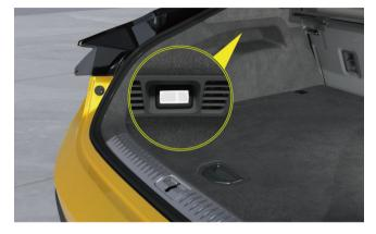
When the tailgate is opened, the boot light will be illuminated automatically. When the tailgate is closed, the boot light will go out automatically.
