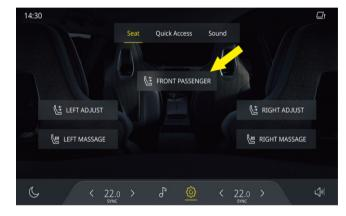
You can tap the 9 icon on rear display and select **Seat** to access the seat settings interface, where the position of front passenger seat can be adjusted by tapping the **FRONT PASSENGER**.
