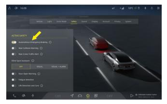
You can tap the @ icon on the CSD and select **Safety** to access the AEB setting interface, where you can tap to turn on or off the AEB.
