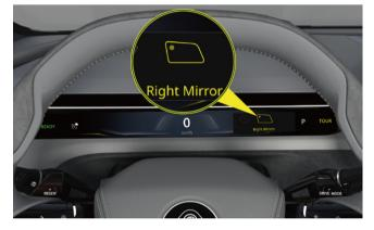
Move the menu/voice button upward to activate the outside wing mirror adjustment. Scroll the right multi-function button left and right to switch to corresponding outside wing mirror.
