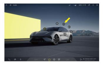
You can tap the cicon on the CSD, and tap the active tail switch to enter the manual control active rear spoiler interface.
