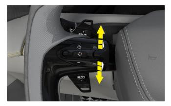
Toggle the following distance button up and down: place your thumb on the lower or upper part of the following distance button, and toggle the knob up or down until a crisp sound is heard.
