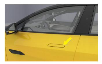
When the walk-up unlock feature is turned off, carrying the key fob and touching the driver's door handle switch can lock or unlock the vehicle.
