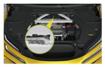
Check the coolant level from time to time to ensure that the level is between the MIN and MAX marks.
