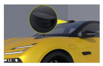
Open **Welcome show** (p.113) and when the vehicle is unlocked, the LiDAR will automatically unfold and fold up.
