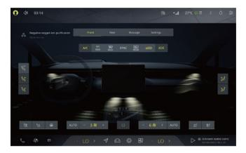
On the A/C control interface, double-tap to turn on the corresponding air flow, and double-tap again to turn it off. Tap and drag the air flow to adjust the air flow direction.
