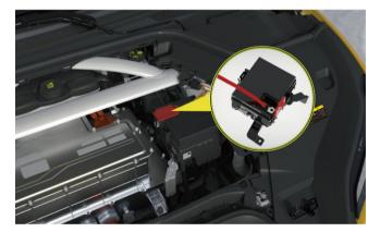
Park the vehicle in a safe area, and open the fuse box cover in the bonnet of the vehicle with dead battery.
