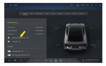
Before replacing the front wiper blade, activate **Settings – Vehicle** – **Windscreen Maintenance** on the CSD, and the front wiper arms will move to the maintenance position.
