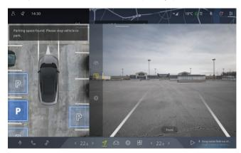
3. When an available parking space is detected, depress the brake pedal to stop the car stably. The driver can get out of the car with valid key and phone carried after clicking the REMOTE PARKING button and hanging into P gear.
