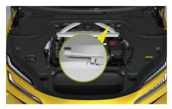
Check the brake fluid level from time to time to ensure that the level is between the MIN and MAX marks.
