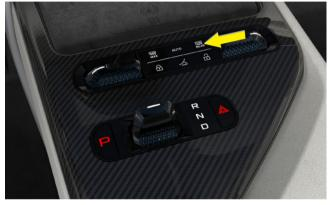
Outside wing mirror heating via tunnel console
