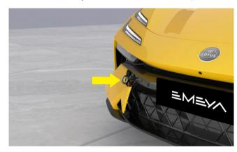
Mounting hole of front bumper towing ring
