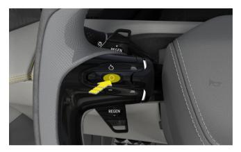
Press the left multi-function button: place your thumb in the middle of the multi-function button, and press the button until there is a crisp sound.
