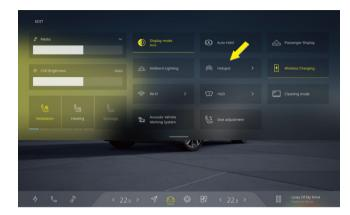
Click the occor icon in the CSD to open the vehicle hotspot setting interface. Enable the vehicle hotspot and enable the Wi-Fi connection of the mobile phone or other devices, then you can find the vehicle hotspot name on the mobile phone or other devices. Tap Connect, and the vehicle hotspot setting is successful.
