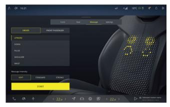
You can tap on the central screen display's air conditioning control interface **Massage** to switch to the front seat massage settings
