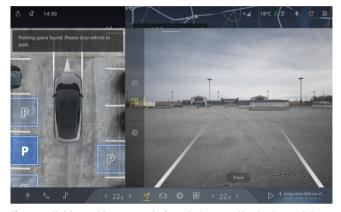
If an available parking space is found, depress the brake pedal to stop the vehicle and tap the IN CAR button.
