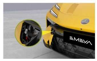
Emergency unlocking via external power supply
