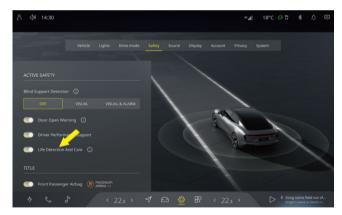
The life detection and care system is enabled by default, and you can choose to enable or disable this function by tapping the loon on the CSD and selecting **Safety**. After this function is disabled,
