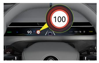
The alarm will be triggered when the vehicle speed exceeds the speed limit recognized by the system; The alarm will be released when the vehicle speed is below the speed limit recognized by the system until a new speed limit is detected.
