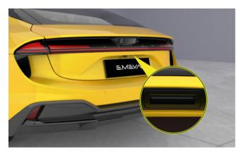
Emergency unlocking via tailgate opening switch
