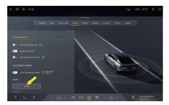
When the vehicle is powered on and the gear lever is in the P position, you can manually unfold all the LiDARs with one touch as needed. The LiDAR cannot be deployed manually in any of the following conditions:
