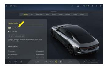
When the ESC and EPB systems are fault-free, you can click @ icon in CSD to select the **Vehicle**, and enable AUTO HOLD.
