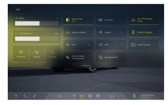
Swipe down on the top of the centre display to open the shortcut panel. Tap the function tab to quickly turn on/off the corresponding
