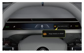
When LKA works, the driver is required to hold the steering wheel with both hands at all times. When the LKA is activated for the first time and the system detects that the driver is not holding the steering wheel, no prompt message will appear on the instrument cluster. If the LKA is activated again in the next period of time, and the system detects that the driver is still not holding the steering
