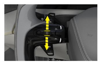
Toggle the left multi-function button up and down: place your thumb in the middle of the lower or upper part of the multi-function button, and toggle it up or down until a click is heard.
