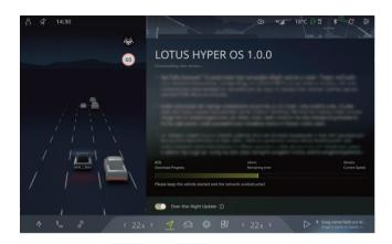
You can open the OTA system upgrade interface by clicking  $\underline{\psi}$  icon at the top of the central display or clicking  $\underline{\emptyset}$  icon and selecting **System** - **Check for update** from the setting interface. The update information field will show the purpose, items, the estimated time required for the upgrade, the impact of the upgrade on the vehicle functions and any notes related to the upgrade.
