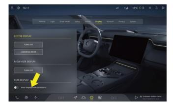
When you want to prevent rear passengers from operating the rear display, you can tap the @icon on the CSD, select **Display**, and then tap **Rear display lock (Child lock)** to turn on or off the rear display locking function.
