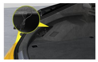
The emergency rope of the electronic lock is placed at the upper hinge of the driver's door.
