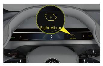
Scroll the menu/voice button to activate the outside wing mirror adjustment. Scroll the right multi-function button left and right to switch to the corresponding streaming mirror.
