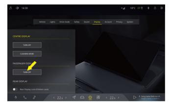
After the vehicle is powered on, you can tap the screen OFF switch or on the screen as required to turn off or activate the passenger screen. You can also click on the icon in CSD, select to **Display**, and click to **TURN ON** or **TURN OFF** switch on this interface to activate or deactivate the passenger screen.
