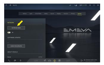
When the network status is poor, you can click the icon @ on the CSD, click **NETWORK RESET** on the **System** setting interface, and restart the vehicle system to reconnect to the network after a period of time.
