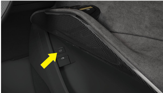
Tailgate switch on driver door
