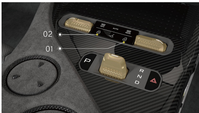
Central lock on tunnel console
