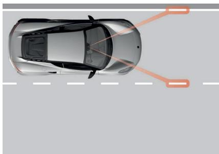
A camera mounted behind the top of the windscreen monitors any available traffic lane markings, comparing the road direction with the steering wheel movement.
