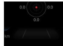
No line markings detected or system in standby.
