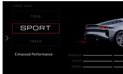
A description of the driving characteristics for the mode selected is shown as well as the level of powertrain, exhaust sound and electronic stability control intervention available, which are represented as illuminated bars at the bottom of the display.
