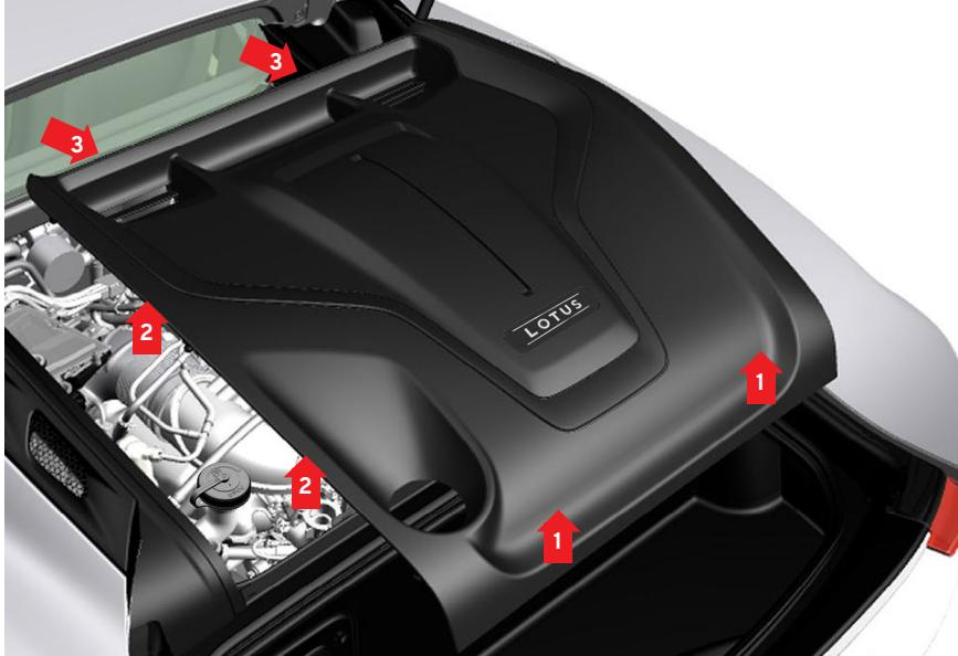
Before closing the tailgate, check that all of the engine compartment panels have been fitted correctly and are secure.
