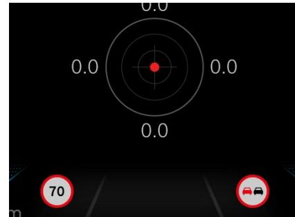
If traffic sign recognition is activated, once the vehicle passes a recognisable road sign, it is displayed as a symbol in the lower centre of the driver display.
