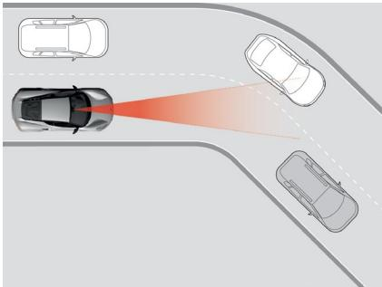
the road surface, dirty road surfaces or unclear lane markings can also significantly reduce camera function when it is used view the road for road sign information.
