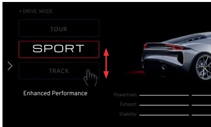
Either move the drive mode switch backwards or forwards again, as required to change to a new mode setting, or press the mode button on the centre display.
