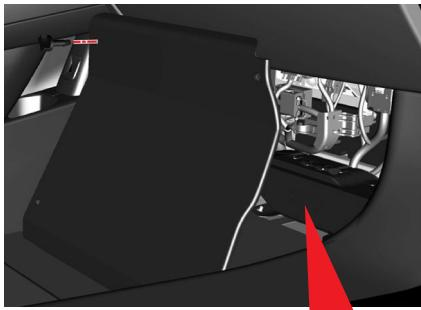
The toe board panel is an occupant crash protection component. Never drive the vehicle without the toe board panel being installed and fitted correctly.
