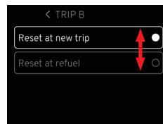
Press  $\triangle$  or  $\text{O}$  to highlight reset option and press  $\text{O}$  to select.
