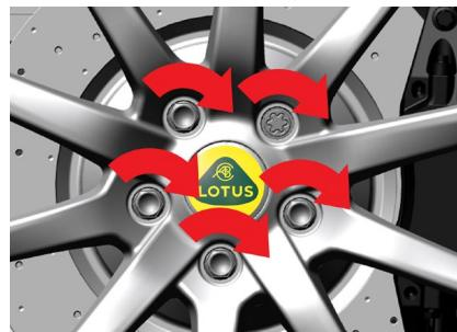
4. Tighten all 5 wheel bolts in a crosswise pattern using the standard extension and (and coded wheel bolt adaptor if locking wheel bolts are fitted).
