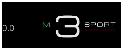
If a paddle is not operated within a 20 second interval then the transmission will return to automatic mode selecting the appropriate gear, which may differ from the gear last manually selected.
