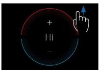
Press and drag up just outside of the display to set 'Hi' temperature.
