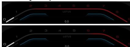
Maximum engine speed is graduated up to a maximum of 6,000 rpm during engine warm up until normal running temperature has been reached, the revised maximum rpm value display in
