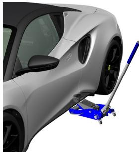
7. Position a suitable jack at the rear lifting point identified by a blue sticker, see page 250, 'Raising the Vehicle'. This will raise both wheels on that side of the vehicle.
