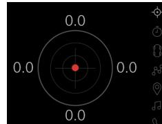
Pressing O displays the maximum g-force values (measured as g), attained during the current drive cycle.
