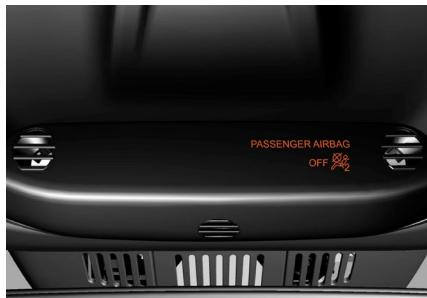
If the occupant classification sensor system detects a group 1 passenger type, the upper console displays a message and a crossed-out child seat symbol informing that the passenger airbag is disabled (will not inflate) in the event of a collision.
