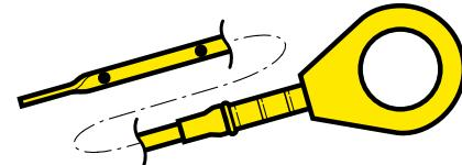
The level should be between the two dots on the lower end of the dipstick.
