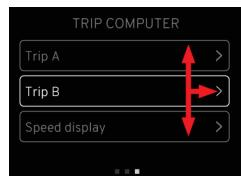
From trip computer menu press  $\triangle$  or  $\text{O}$  to highlight Trip B and press  $\text{O}$  to select.
