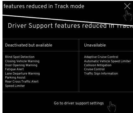
Tap the close button on the top right-hand of the display to return to the previous screen.
