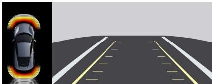
The camera will automatically activate at any speed when reverse gear is selected, or manually using the centre display screen.
