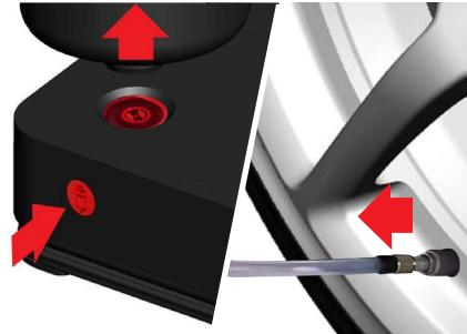
17. Disconnect the compressor connector from the 12V auxiliary power socket, press the button on the side of the compressor to detach the tire sealant bottle and refit the tire valve cap.
