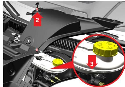
**Brake/Clutch Fluid Level Check**
