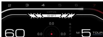
The performance shift lines and shift blocks will slowly flash and **SHIFT** will be displayed as engine speed continues to increase, indicating to the driver that the ideal shifting point has now been reached.
