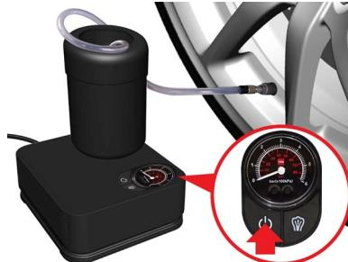
15. Press the
