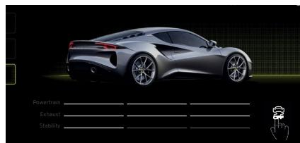
All stability level bars will extinguish indicating that ESC is not available (except for ABS and HBA functions).
