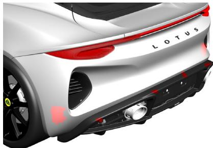
Location of rear radar units. Keep the area shown clean on both the left and right-hand sides of the vehicle.
