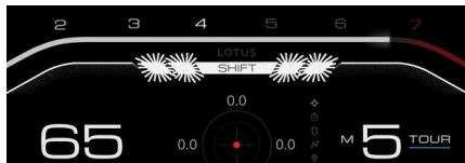
If the prompt to shift gear is ignored and the engine speed exceeds the final shift point, the performance shift lines and blocks will flash faster.
