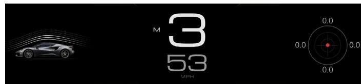
With the driver's display in track mode, the track widget selected is shown on the left of the screen and the other menu option selected is shown on the right.
