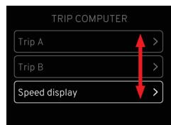
From trip computer menu press  $\triangle$  or  $\text{O}$  to highlight Speed display and press  $\text{O}$  to select.
