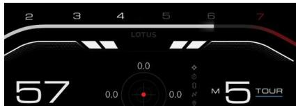
Continued increase in engine speed whilst remaining in the same gear will illuminate the third, inner level shift blocks.
