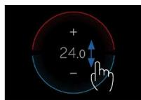
Press and drag up or down inside the display to change the temperature.
