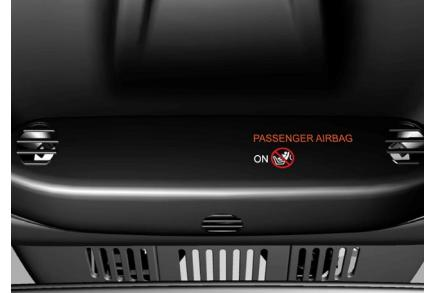
If the occupant classification sensor system detects a group 2 passenger type, the upper console displays a message and a crossed-out child seat symbol informing that the passenger airbag is enabled (may inflate in the event of a collision).
