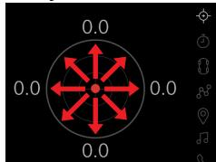
The current directional g-force experienced by the vehicle is indicated by the red dot as it moves across the area within the circles, which represent the different levels of g-force.
