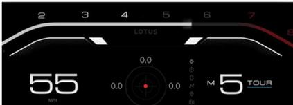
If engine speed continues to increase whilst remaining in the same gear, the second shift level will be reached, illuminating the outer shift blocks.
