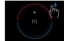
Press and drag up just outside of the display to set 'Hi' temperature.
