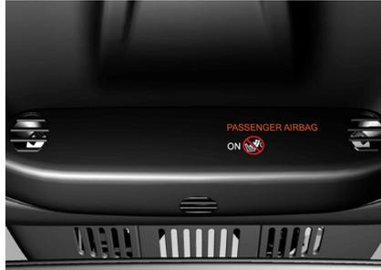
The upper console also shows a message and symbol informing that the passenger airbag is activated.
