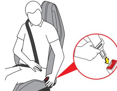
1. Sit erect and fully back in the seat. Hold the seat belt tongue, pull it across the body and withdraw the belt from the retractor.
