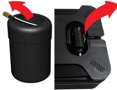
7. Remove the electrical connector/cable from the compressor stowage compartment and the transparent airline hose from the tyre sealant bottle.
