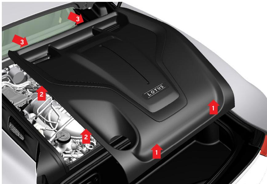
Before closing the tailgate, check that all of the engine compartment panels have been fitted correctly and are secure.
