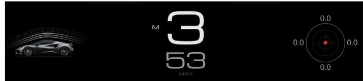
With the driver's display in track mode, the track widget selected is shown on the left of the screen and the other menu option selected is shown on the right.
