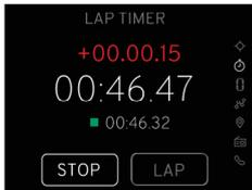
If a best lap time is available when a new lap is registered, then the time difference between the previous lap time and the current best lap time for the session is displayed for 10 seconds.
