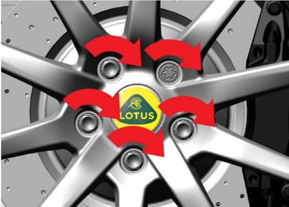
4. Tighten all 5 wheel bolts in a cross-wise pattern using the standard extension and (and coded wheel bolt adaptor if locking wheel bolts are fitted).
