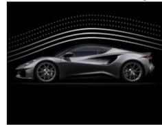
Press or to display the current downforce. The number of illuminated airstream lines above the vehicle increase as downforce increases.
