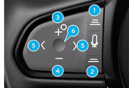
Cruise and adaptive cruise control are operated using the switches on left-hand side steering wheel keypad.
