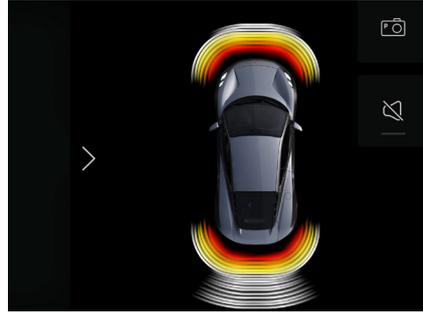
When active, an image of the vehicle is shown in the centre display, sensor fields indicate any objects that are detected and their proximity relative to the vehicle.
