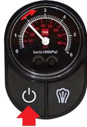
25. Release excessive tyre pressure by pressing the
