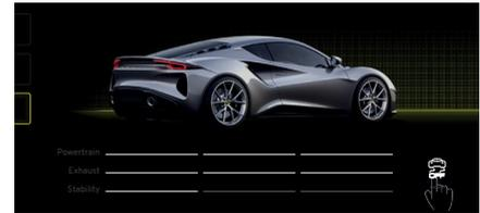
All stability level bars will extinguish indicating that ESC is not available (except for ABS and HBA functions).
