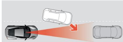
The radar unit may be late to detect vehicles at close distance, such as a vehicle that drives in between your vehicle and the vehicle in front.
