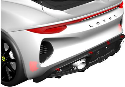
Location of rear radar units (if fitted). Keep the area shown clean on both the left and right-hand sides of the vehicle.
