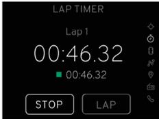
With the LAP button highlighted, pressing **O** again stops the timer and records the lap time. If this is the first lap, then it will be recorded as the current best lap time.
