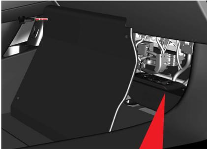
**⚠ WARNING:** The toe board either not installed or incorrectly fitted could result in unbelted front passenger being at risk of injury to their upper leg area in the event of unbelted crash situation.
