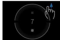
Press and drag outside display to set fan speed to '7'.
