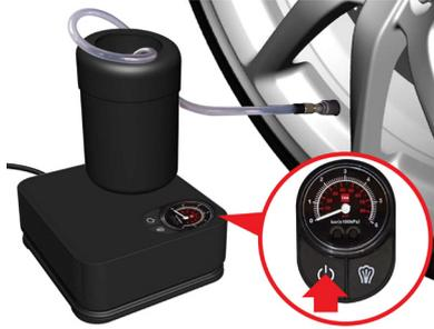
15. Press the
