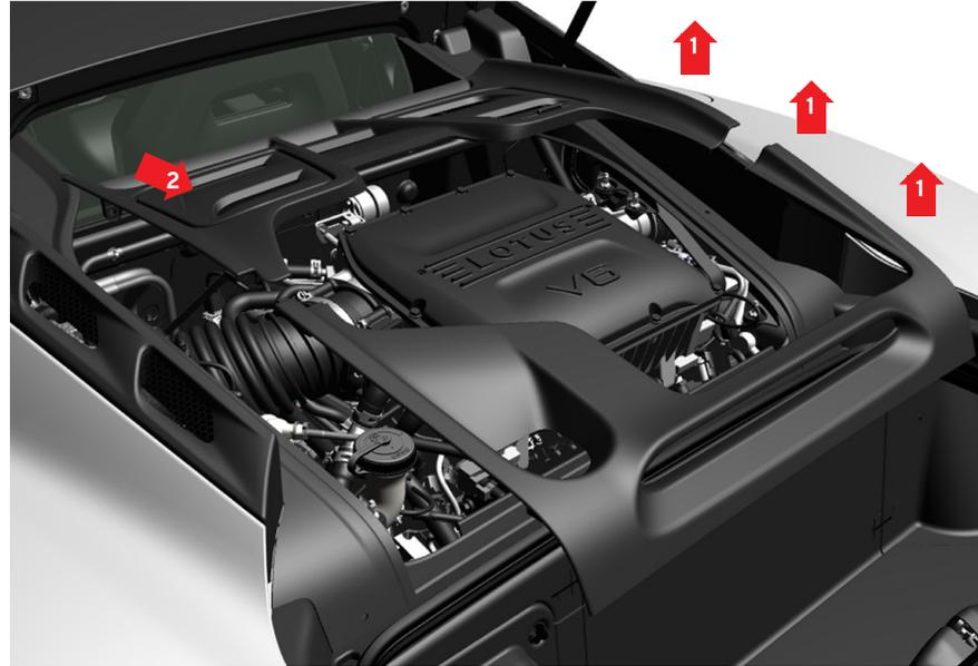
**📖 NOTE:** To prevent accidental damage to the panels, place them in a safe area with the fixings facing downwards.
