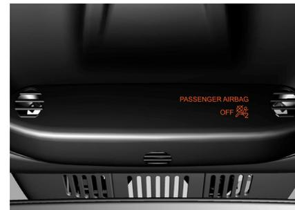
The upper console also shows a message and symbol informing that the passenger airbag is deactivated.
