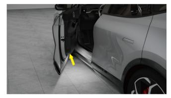
When the external environment is dim, the floor lights will be illuminated automatically as the doors are opened and they will automatically go out as the doors are closed.
