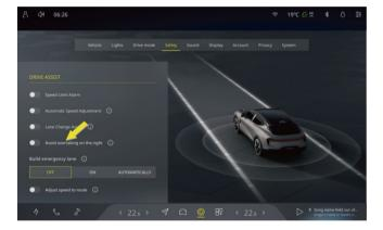
Click the @ icon on CSD and select **Safety** to enter the driving assist setting interface, turn on or off the avoid overtaking on the right.
