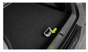
A boot storage box is provided under the boot floor, which can be used to store driver's tools.
