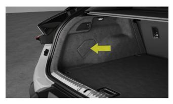
Remove the boot storage box to find the rear electric fuse box.
