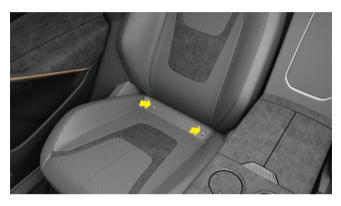
I-Size anchorages are located in the two rear outer seats, and the I-Size logo is printed on the cover of the anchorages.
