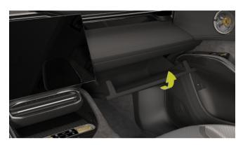
Push the glove box back to lock it properly, and the glove box indicator will go out automatically.
