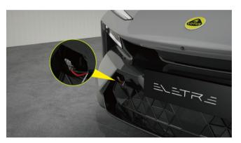
Emergency unlocking via external power supply
