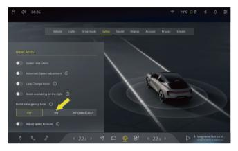
Click the @ icon on CSD and select **Safety** to enter the driving assist setting interface, turn on or off the build emergency lane.
