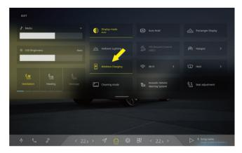
Swipe down from the top of the CSD to open the quick panel, and click Wireless Charging to turn this function on or off.
