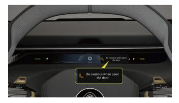
If DOW detects a target and there is a risk of collision when the door is being opened, the indicator on the outside mirror will be illuminated or flash, accompanied by an audible alarm, and images and text alarm signals will pop up on the instrument cluster.
