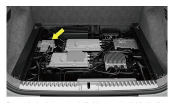
Remove the boot storage box to find the rear main distribution fuse box.
