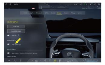
After you turn on the **Rear display lock** function, tapping the rear display will briefly light up the screen, where the method of reopening the rear display will appear. If you do not operate for a period of time, the rear display be will automatically locked.
