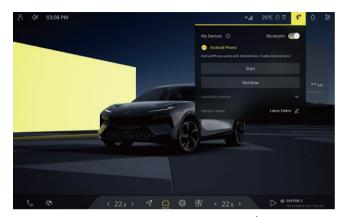
After Android Auto is connected, there will be an ♠ icon in the upper left corner of the CSD, and the ♠ icon in the device list will light up.
