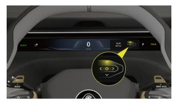
Streaming mirror adjustment interface via steering wheel button\*
