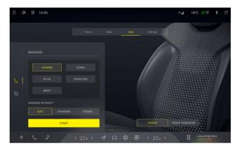
You can click **Massage** in the A/C control interface on central display screen to switch to front seat massage setting interface, and then select the massage modes and massage intensities according to your needs.
