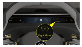
Scroll the menu/voice button to activate the outside wing mirror adjustment. Scroll the right multi-function button left and right to switch to the corresponding streaming mirror.
