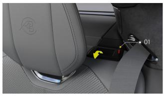
The locking device is located on the outer side of the head restraint
