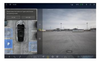
4. Follow the instructions to release the brake pedal and steering wheel, and start to automatically drive into the parking space.
