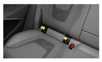
I-Size anchorages are located in the two rear outer seats, and the I-Size logo is imprint on anchorage connection points.
