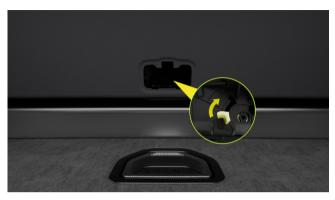
Emergency unlocking of tailgate control lever
