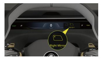
Move the menu/voice button upward to activate the outside wing mirror adjustment. Scroll the right multi-function button left and right to switch to corresponding outside wing mirror.
