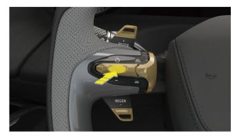
Press the left multi-function button: place your thumb in the middle of the multi-function button, and press the button until there is a crisp sound.
