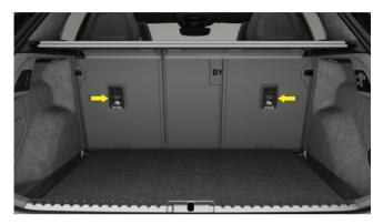
The top tether anchorages of the child safety seat is located behind the rear seat backrest.
