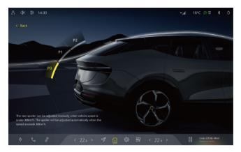
You can manually adjust the active rear spoiler by clicking on different gears.
