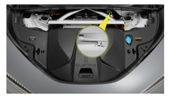
Check the brake fluid level from time to time to ensure that the level is between the MIN and MAX marks.
