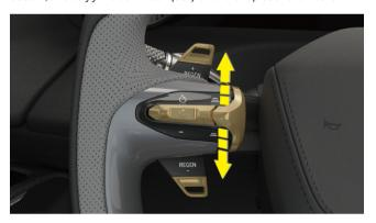
Toggle the following distance button up and down: place your thumb on the lower or upper part of the following distance button, and toggle the knob up or down until a crisp sound is heard.
