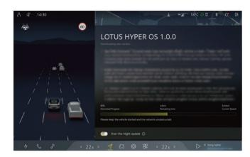
You can open the OTA system upgrade interface by clicking  $\underline{\psi}$  icon at the top of the central display or clicking  $\underline{\mathfrak{G}}$  icon and selecting System - Check for update from the setting interface. The update information field will show the purpose, items, the estimated time required for the upgrade, the impact of the upgrade on the vehicle functions and any notes related to the upgrade.
