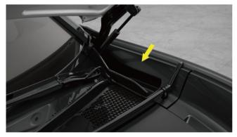
3. Push the locking lever of the charging port cover backward to unlock the charging port cover, then pull it out from the gap and open the charging port cover.
