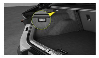
When the tailgate is opened, the light in the boot will be illuminated automatically; when the tailgate is closed, the light in the boot will go out automatically.
