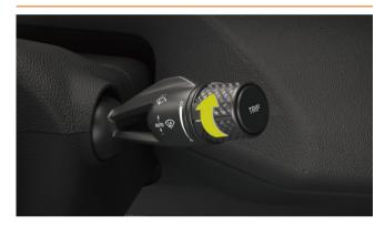
The sensitivity of the induced rainfall can be adjusted by turning the sensitivity scroll wheel of the RLSM upward and downward. The higher the sensitivity when turning the scroll wheel upward, the shorter the wiping interval will be. Conversely, the lower the sensitivity when turning the scroll wheel downward, the longer the wiping interval will be.
