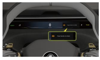
When LKA works, the driver is required to hold the steering wheel with both hands at all times. When the LKA is activated for the first time and the system detects that the driver is not holding the steering wheel, no prompt message will appear on the instrument cluster. If the LKA is activated again in the next period of time, and the system detects that the driver is still not holding the steering
