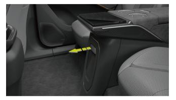
The rear tunnel console pocket is located under the rear seat centre armrest, which can be opened by pulling it out.
