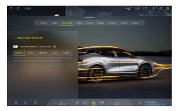
You can choose to activate or deactivate the Variable Traction Control (VTC) in Track mode. If the VTC is activated, you can set the traction control level.
