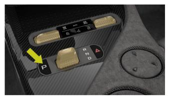
After the vehicle is parked, press the P button, the gear switches to P gear, and the electronic parking brake is automatically activated.
