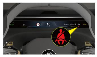
The reminder in the instrument display and a relevant message in the CSD, alerts unbelted occupants to wear a seatbelt. If all seat belts are worn properly but the reminder and alarm do not extinguish, then contact your Lotus retailer.
