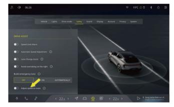
Click the @ icon on CSD and select **Safety** to enter the driving assist setting interface, turn on or off the adjust speed to route.
