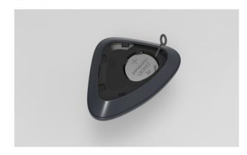
4. When installing the cover plate on the back of the key, press hard against the clip to tighten it.
