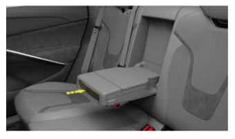
Press the front end of the cup holder to make the cup holder automatically pop out.
