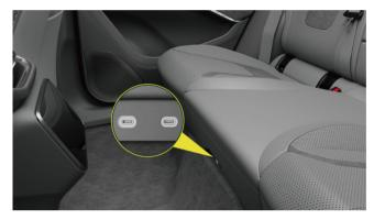
There are two USB-C ports in the lower centre of the rear seat cushion, which can be used by passengers for charging.
