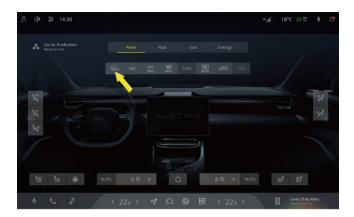
Click the **TEMP** in the CSD to switch to the climate control interface where you can activate or deactivate the defrosting/defogging function of the streaming mirror to remove rain, water mist or ice and snow from the camera.
