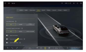
You can click on the @ icon on the CSD screen and select **Safety** to manually turn on or off the **Lane Change Assist** switch.
