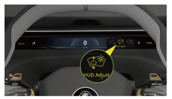
Press the right multi-function button left and right to select the HUD ON/OFF, height, brightness, and snow mode respectively.
