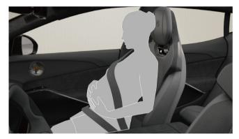
The diagonal section of the belt should wrap over the shoulder and then be routed between the breasts and to the side of the abdomen. The lap belt portion of the belt should be kept as low as possible under the abdomen and it must not be allowed to ride upward. Make sure that the seat belt has no slack and is not twisted.
