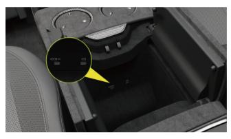
There are two USB-C ports in the rear central armrest box, which can be used by passengers for charging.
