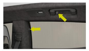
Coat hooks are installed on both sides of the rear B-pillar and above the door for passengers to place clothes or hats.
