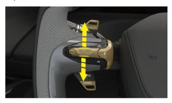
Toggle the left multi-function button up and down: place your thumb in the middle of the lower or upper part of the multi-function button, and toggle it up or down until a crisp sound is heard.
