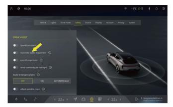
Click the  $\circ$  icon on CSD and select **Safety** to enter the driving assist setting interface, turn on or off the automatic speed adjustment.
