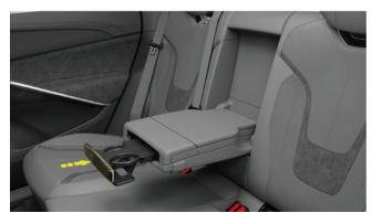
When the rear cup holder is not in use, push the cup holder back to lock.
