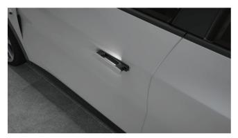
When the ambient light outside the vehicle is insufficient, the handlebar light will be illuminated to illuminate the inside of the door handle for the convenience of vehicle unlocking, and then it will be automatically extinguished after a period of time.
