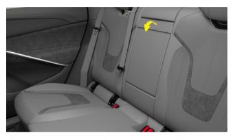
The centre armrest is installed in the middle of the rear seat backrest, which can be turned down and pulled out for use, and turned up and pressed back into the backrest for closing.
