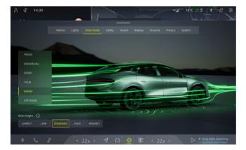
In this interface, you can set the drive mode, and in some driving modes, you can set the body height. The driving mode includes track mode\*, individual mode, sport mode, tour mode, range mode and off-road mode.
