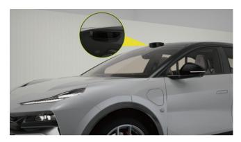
Open **Welcome show** (p.107) and when the vehicle is unlocked, the LiDAR will automatically unfold and fold up.
