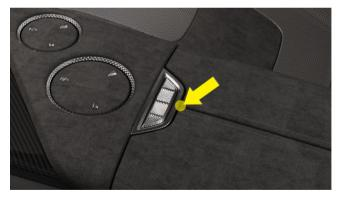
After the armrest is closed, the charging cable or data cable can be extended from the shown position.
