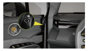
The emergency rope of the electronic lock is placed at the upper hinge of the driver's door.
