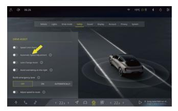
Click the @ icon on CSD and select **Safety** to enter the driving assist setting interface, turn on or off the automatic speed adjustment.
