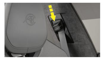
Press and hold the release switch to move the seat belt shoulder height adjuster up and down, which can be adjusted to the proper position according to your requirements so that the seat belt can fit the shoulder better.
