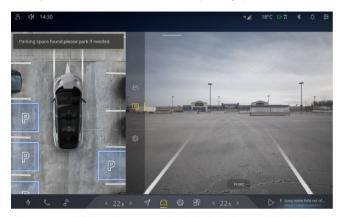
When an available parking space is detected, depress the brake pedal to stop the car stably. The driver can get out of the car with valid key and phone carried after clicking the REMOTE PARKING button.
