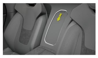
The rear seat backrest pocket is located in the centre of the rear seat backrest, and is pushed down to the bottom lock; Press again and close automatically.
