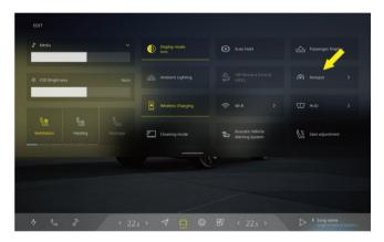
Click the occasion in the CSD to open the vehicle hotspot setting interface. Enable the vehicle hotspot and enable the Wi-Fi connection of the mobile phone or other devices, then you can find the vehicle hotspot name on the mobile phone or other devices. Tap Connect, and the vehicle hotspot setting is successful.
