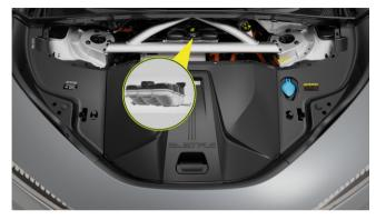
Check the coolant level from time to time to ensure that the level is between the MIN and MAX marks.
