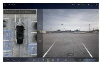
3. If an available parking space is found, depress the brake pedal to stop the car stably and click the **IN CAR** button.
