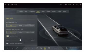
In this interface, the drive assist, active safety and passenger safety can be set.
