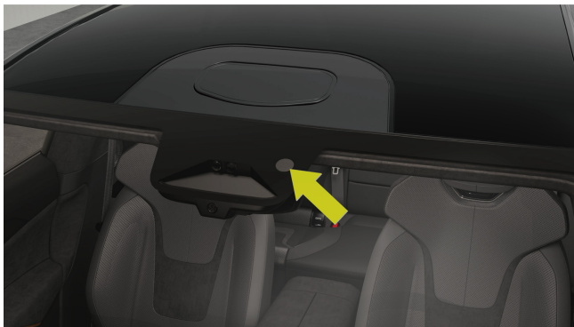
Modul for lysregnsensor (RLSM)
